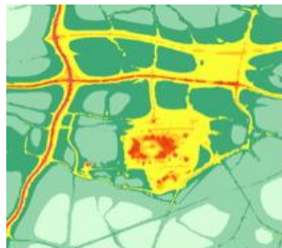
Modelled NO 2 concentrations around Heathrow, 2002 base case (µg/m 3 ) [From "Adding Capacity at Heathrow Airport – Air Quality Studies for Heathrow", 2007]
