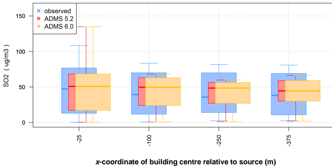
Figure 5 – Box and whisker plot of model results, variation with x-coordinate of building centre relative to source (y-coordinate = 0).
