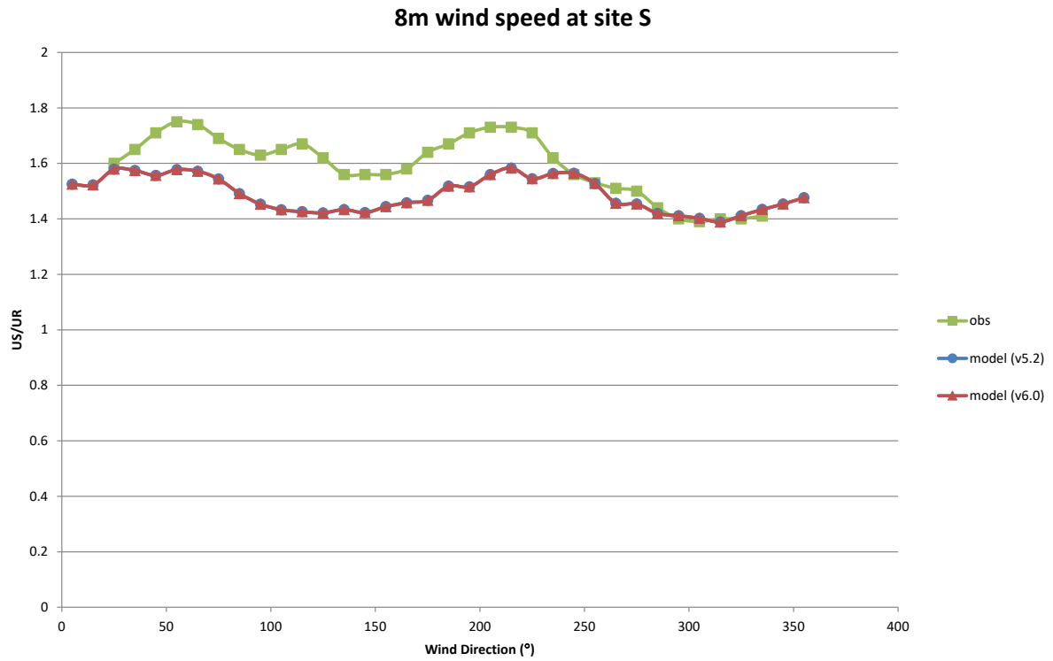
Figure 3 - Comparison of 8 m wind speed at the summit site S
