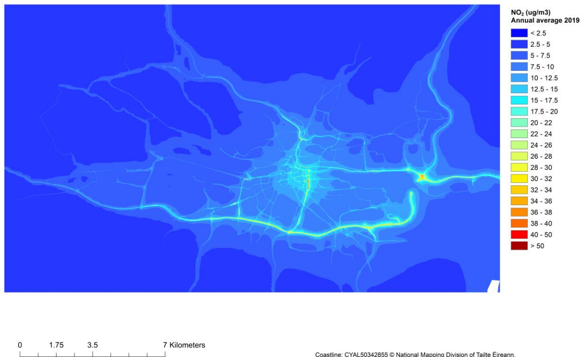
Figure F.4 – Coupled system annual average NO 2 city pollution map for 2019 of Cork; transition to exceedance of AQSR limit (40 µg/m 3 ) shown in bright red .
