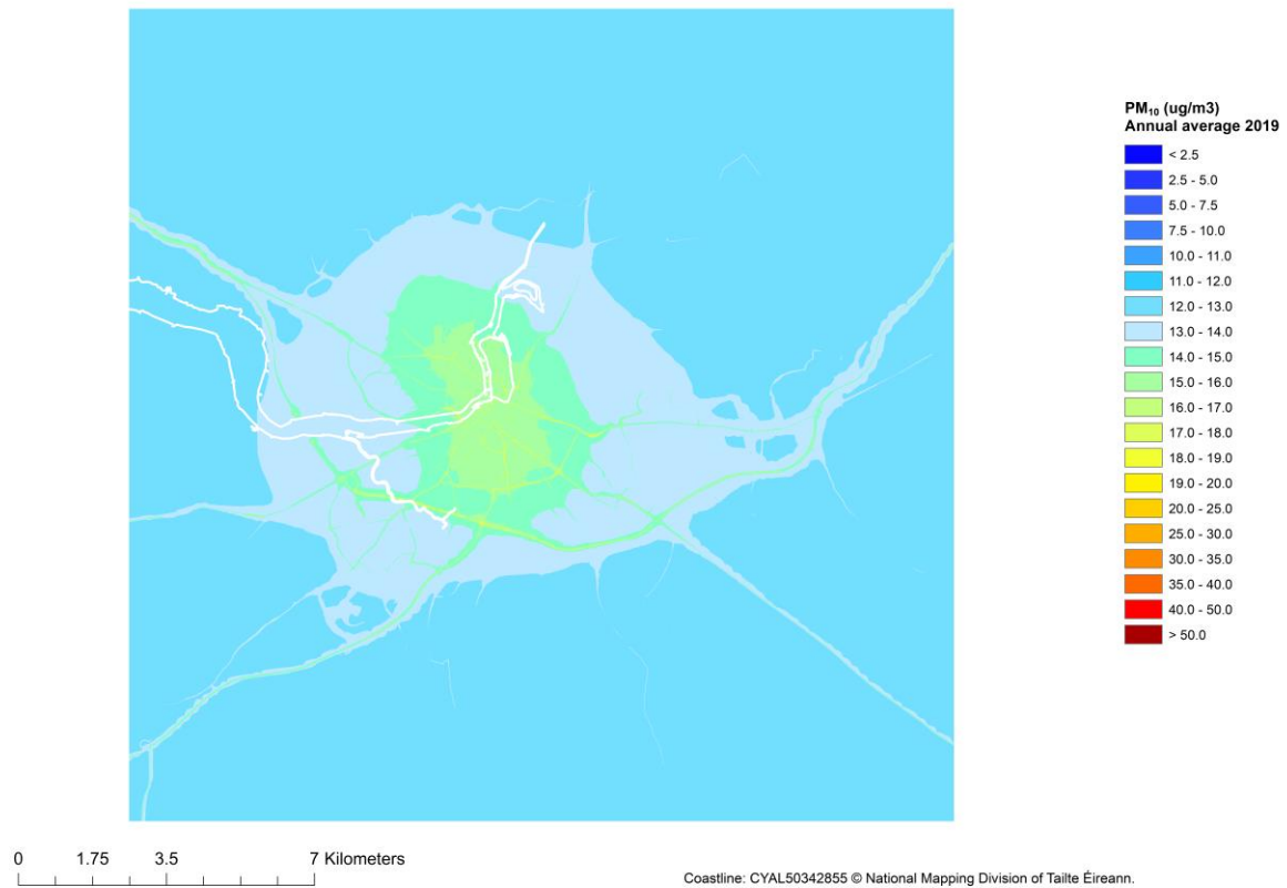
Figure F.13 – Coupled system annual average PM 10 city pollution map for 2019 of Limerick; transition to exceedance of AQSR limit (40 µg/m 3 ) shown in bright red .
